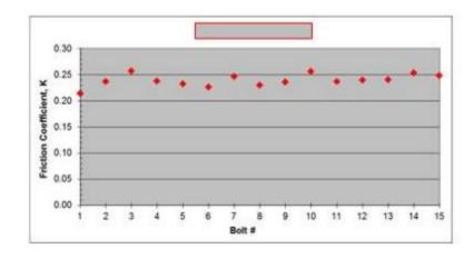
The torque required to achieve 4,941 lb bolt tension (75% of the 6,580 lb proof load), and resulting calculation of  $\mu_{tot}$  are summarized below. The calculation of torque coefficient K (from T=KDF where T=torque, D= bolt diameter and F=bolt tension ) is also included for reference.
