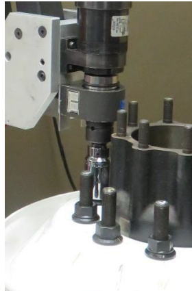
Figure 3: Torque-Angle to Failure Test Setup
