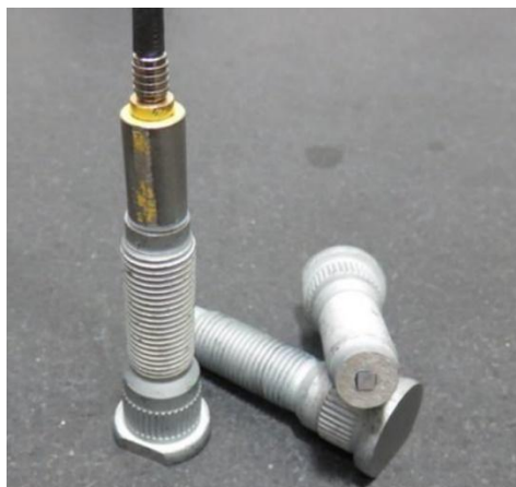
Aluminum Wheel and Wheel Studs Ground and Sensored for Ultrasonic Testing
